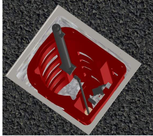
Figure 87: disconnect the cylinder
