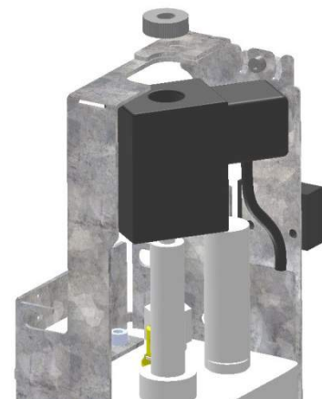
Figure 103: Remove the solenoid valve
