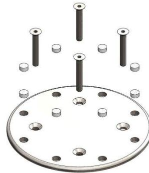
Figure 5: Top plate with screws and light diffusers
