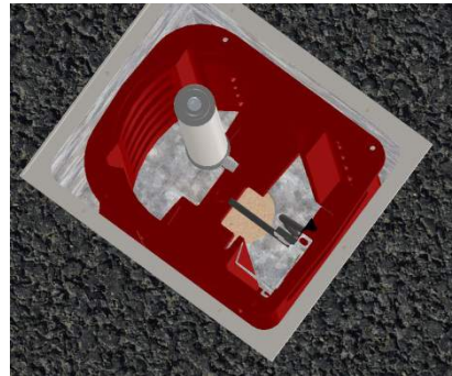
Figure 81: disconnect the cylinder
