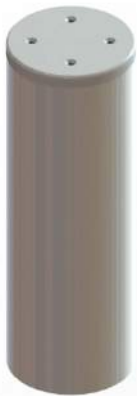
Figure 4: Bollard's covering (top plate and sleeve)
