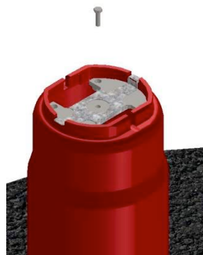
Figure 85: remove the central screw that holds the cylinder
