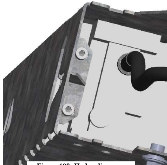
Figure 100: Hydraulic pump bottom assembling screws
