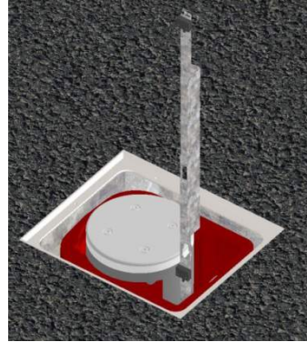
Figure 83: Removing components bracket
