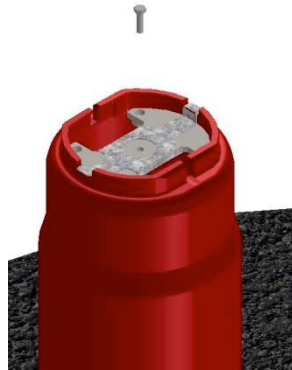
Figure 93: remove the central screw that holds the cylinder
