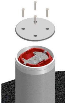
Figure 54: Screws and top plate removing
