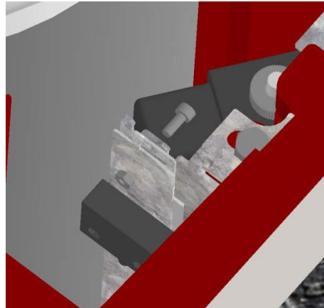
Figure 90: Unscrew the components bracket assembly screw
