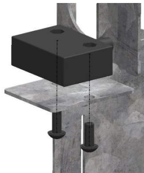
Figure 84: Limit-switch sensor assembling
