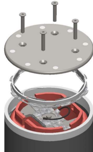
Figure 70: LED light disassembly
