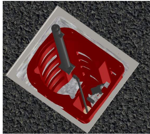
Figure 95: disconnect the cylinder
