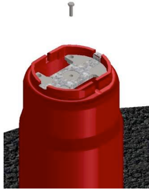
Figure 79: remove the central screw that holds the cylinder
