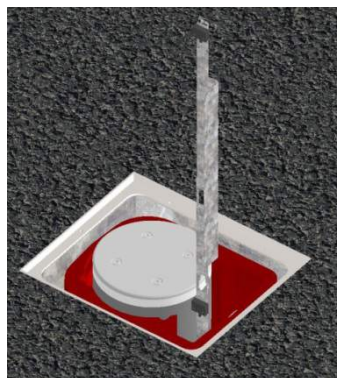
Figure 91: Removing components bracket
