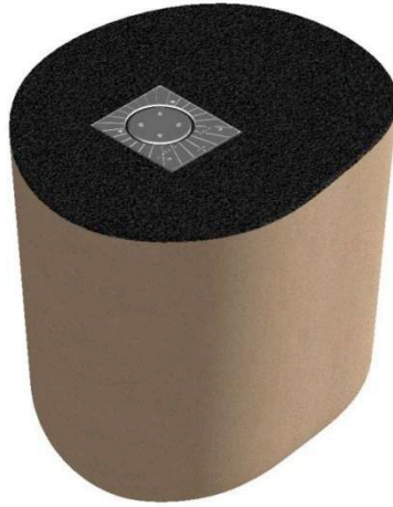
Figure 32: Finished top layer completed with asphalt
